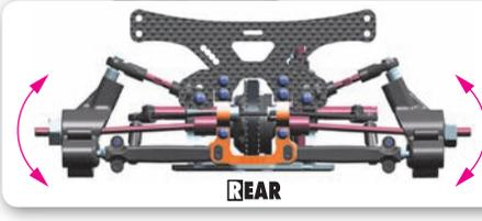
When the bars are set, verify that both sides move at the same time. If they do, the bars are set up correctly. If not, make sure that both downstops are the same and that the bar wire is flat.
