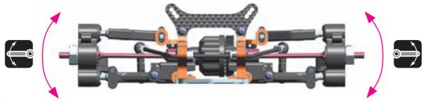
When the bars are set, verify that both sides move at the same time. If they do, the bars are set up correctly. If not, make sure that both downstops are the same and that the bar wire is flat. If the sides still do not move at the same time, adjust the length of the bar holders. **DETAIL**
