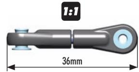
Note the 90° angle difference between the ball joints
