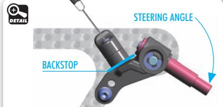
The adjustable backstops are used to limit the steering angle. Adjust the backstop with the set-screw to achieve the maximum steering angle needed. Adjust the steering angle on both L & R sides to the same amount.
